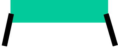
Figure 6. Splayed Pins Required by Integrated Circuit Insertion Tools
