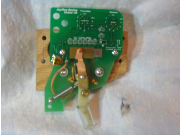
Modified JayGee Racing Linear 200 trigger assembly with shortened trigger travel
