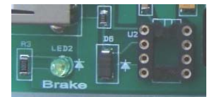
Control chip sockets enable user installation of new throttle and brake profiles as they are released
