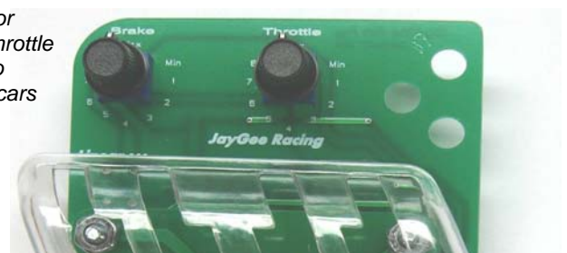
Control chip sockets enable user installation of new throttle and brake profiles as they are released
