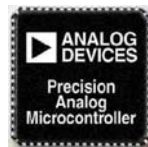
Programmable control chips convert analog pot settings to precise timing pulses
