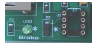
Brake profile chip sockets enable user installation of new profiles as they are released
